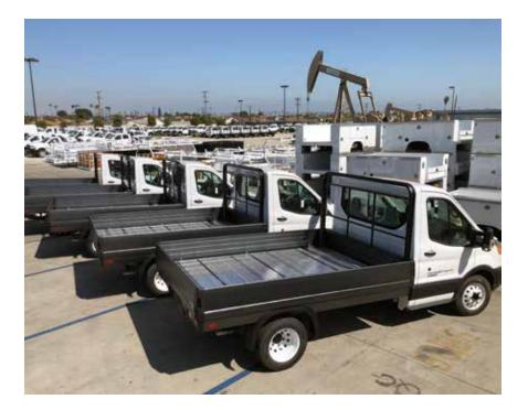
free loading and hauling of freight, merchandise, or other equipment the job demands. Made from industrial grade aluminum, Tri-Gate beds are strong and durable, yet light in weight, and corrosion-resistant.
