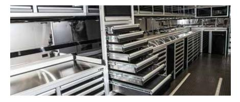
allows the unit to survive the rigors of transport while also cutting valuable weight and increasing payload, because lightweight doesn't have to mean light-duty. To finish each drawer, the frame, top tray, and drawer front are powder coated to provide a long-lasting, aesthetic finish of the customer's choice. CTech also just recently introduced a new 'Full-Bank' locking mechanism for its tool drawers, allowing the user to lock and unlock an entire drawer bank with just one turn of a key.
